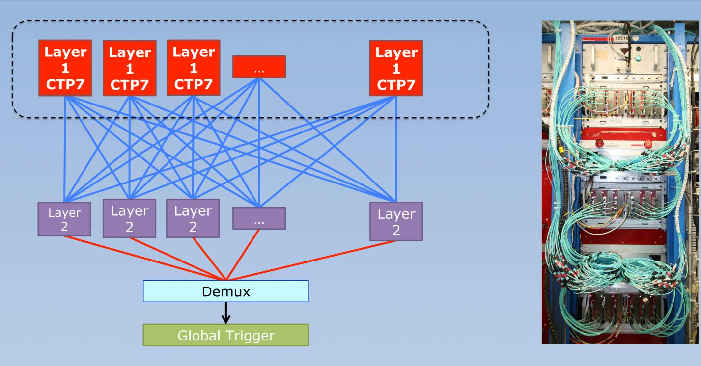
(Above) CMS Calorimeter Stage-2 Layer-1 Trigger, implemented using CTP7 cards.
