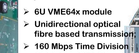
Multiplexed (TDM) and **Bi-Phase Mark (BPM)** encoded channels; One TTC-LKr module
