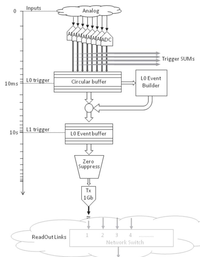
CREAM is 6U VME64x module, its data processing flow with multiple levels of triggering is illustrated here and can be summarised as follows:
