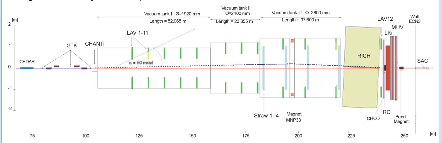
The high resolution Liquid Krypton (LKr) calorimeter of the former NA48 experiment [2], together with other detectors, provides a photon-veto with hermetic coverage from zero out to large angles from the decay region. The study of an upgraded LKr readout system began in 2009.
