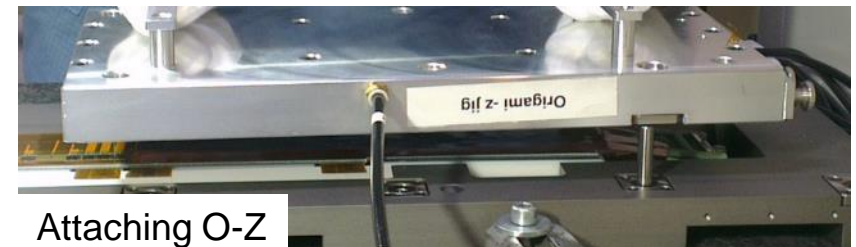
OCE already glued onto sensor, applying glue onto O-Z
