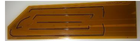
Applying glue onto pitch adapter
