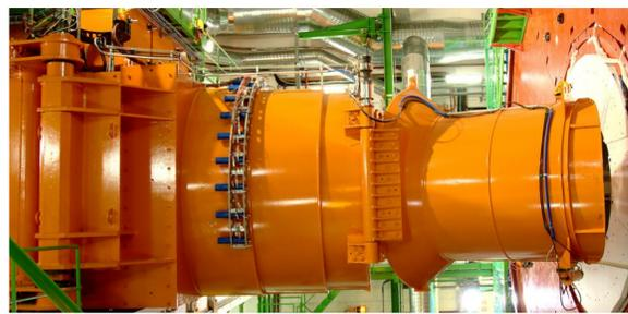
40 BHM detector units (blue cylinders) are installed on the CMS rotating shielding, 20 on each end, at a radius of 1.8 m from the beam pipe and a distance of 20.6 m from the Interaction Point. Their front face is pointed towards the incoming beam in order to be sensitive to beam background.
