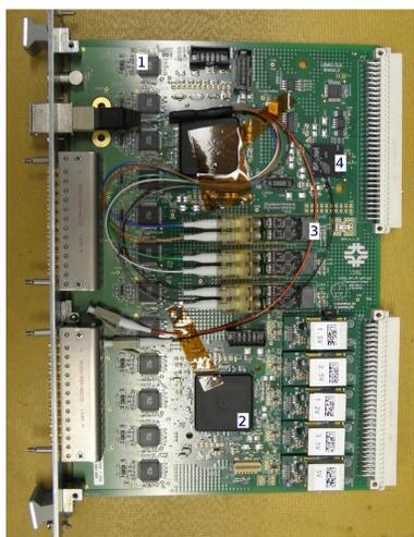
The Front-End electronics are based on the QIE10 ASIC, which provides high dynamic range charge integration and digitization and a 6 bit TDC with 500 ps resolution [3].
