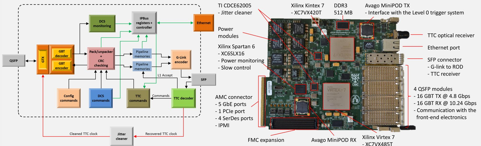
The TilePPr board has been designed in a double mid-size AMC form factor which can be operated in a ATCA carrier or in a  $\mu$ TCA crate. The PCB stack-up is a 16 layer design based on NELCO 4000-13 SI dielectric material to get low losses at high frequency, where 8 layers are dedicated for power and ground planes and 8 layers for signals. The total PCB thickness is 1.6 mm, compliant with the AMC standard.
