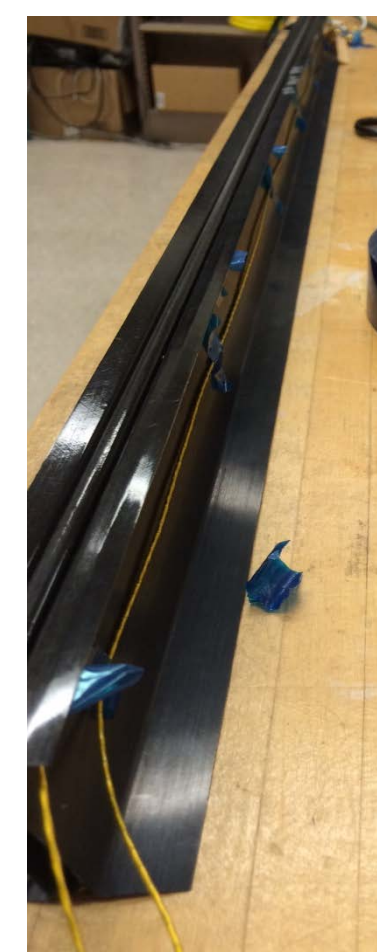
Figure 6, 7. (Left, Below) Modules will be mounted on Carbon-Fiber I-beam (LBNL) and provide reasonable testing environment for Transmission line cross-talk.
