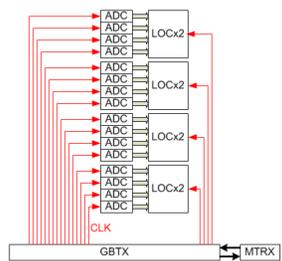
The block diagram of the clock distribution
