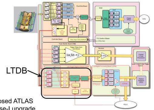
The architecture of the proposed ATLAS LAR trigger electronics in Phase-I upgrade
