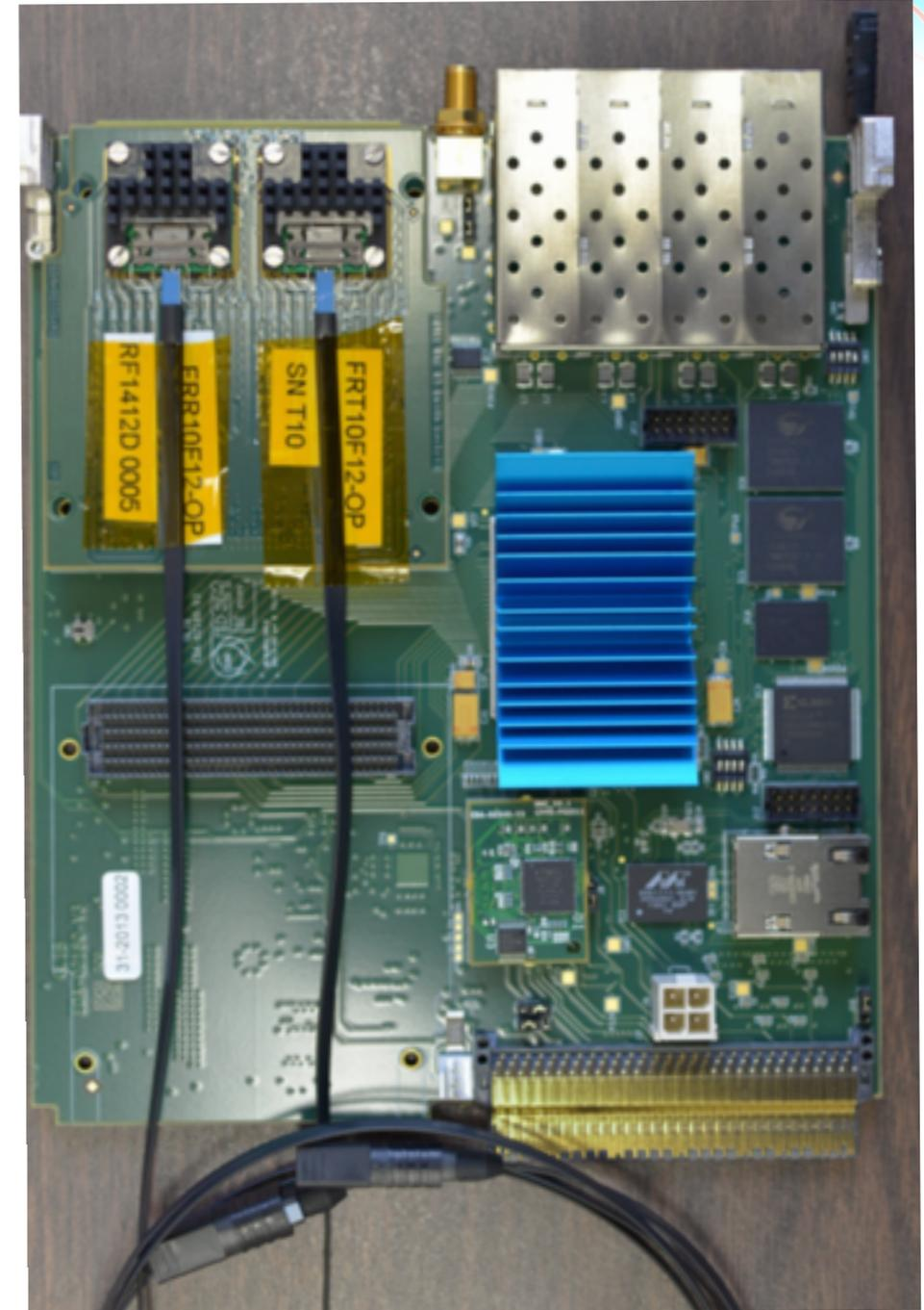
**GLIB w. 2 x FITEL Tx module mounted on FMC (requires adapted Rx)**
