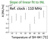
Temperature dependence is obtained to be small for both DNL and INL from -10 deg C to 60 deg C.
