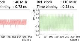
Measured DNL; is < 0.5 LSB for all counts up to  $\sim 300$ . Performance is affected by the time differences between signal paths, which are 100-200 ps in the demonstrator.
