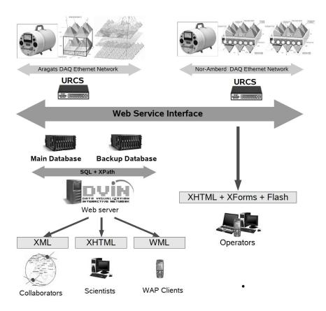
**Figure 1.** The figure represents a layout of the new ASEC data acquisition system. Several detector arrays are operating at Nor-Amberd and Aragats research stations. The detectors are controlled by URCS which are installed on each station. The data dissemination and detector control is facilated by web services. The DVIN is used to distribute the data to end users.
