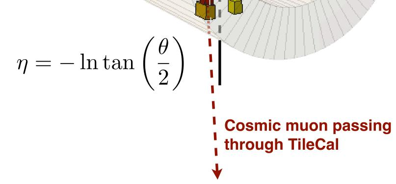
Event display: During commissioning runs with cosmic muons, the event display is an important instrument to both confirm the quality of triggered events and to quickly spot major detector malfunctions. Event data from all sub-detectors taking part in the data taking is reconstructed by a dedicated processing task and combined in the display.
