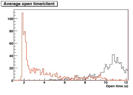
The red histogram shows the distribution of file open times for <23 simultaneous clients. The black histogram shows the case for >23 clients. This shows how the DPM response time changes under load. N.B. all clients start with a file open call within 1s in our tests.
