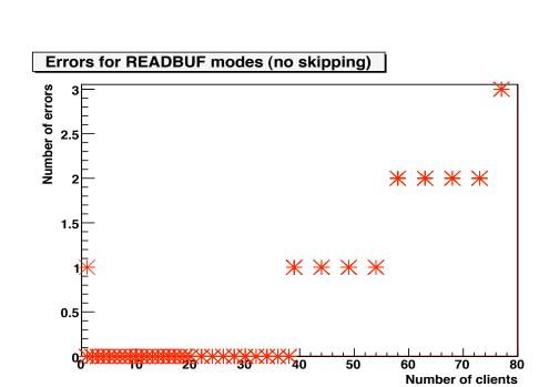
In the case where the access to the file is sequential and with a buffer size of 1MB, a small number of errors were recorded for RFIO\_READBUF mode. This is a significant improvement compared to versions of DPM before 1.6.5 where the error count grew rapidly after ~20 clients
