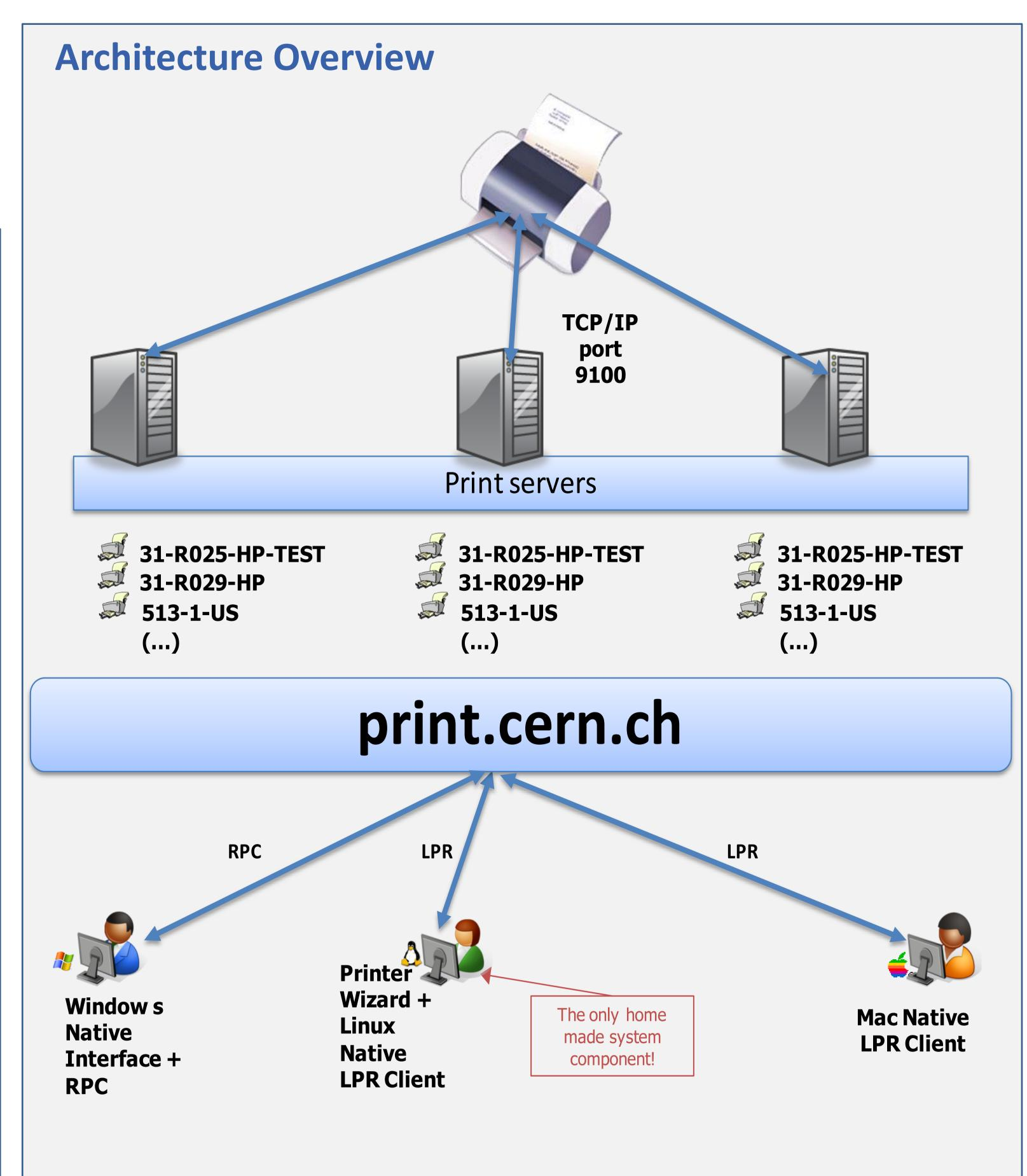
The architecture of CERN printing service consists of three servers configured in the same way. Each server has queues configured for all printers and hosts SOAP interfaces which allow to reconfigure the printer queues. The initial configuration for each driver must be set by an administrator:
