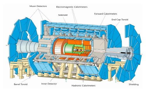
Figure 1. Schematic of ATLAS detector.
