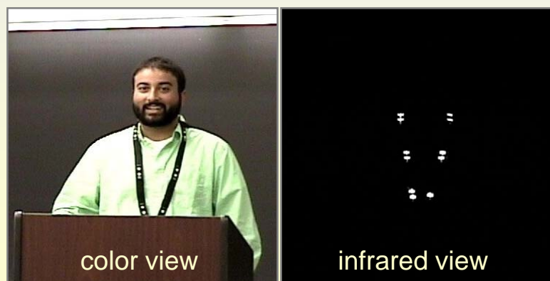
new necklace with super-bright IR LEDs
