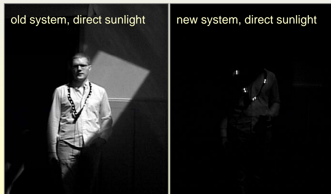
new necklace with super-bright IR LEDs
