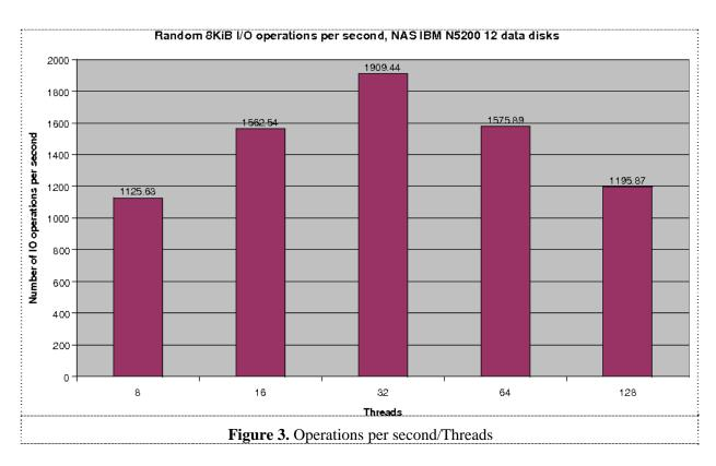
With more than 64 threads disks start saturating and the number of operations starts dropping.
