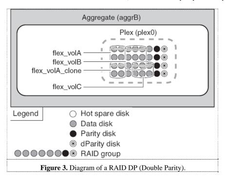
RAID-DP improves standard RAID 6 performance due to the behavior of the storage controller software. All file system requests are first written to the battery backed NVRAM to ensure there is no data loss should the system lose power. Blocks are never updated in place, so when incoming write
