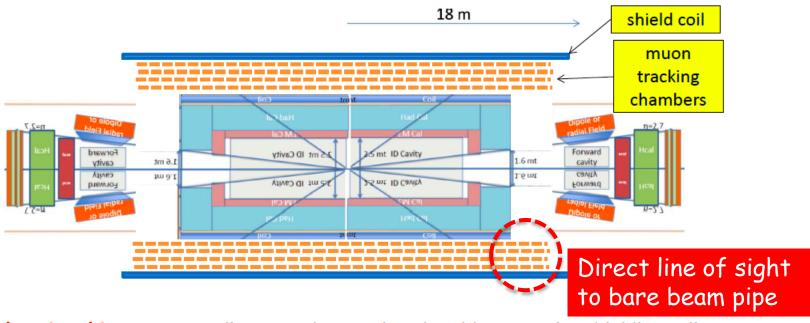
Twin Solenoid: a 6 T, 12 m dia x 23 m long main solenoid + an active shielding coil
