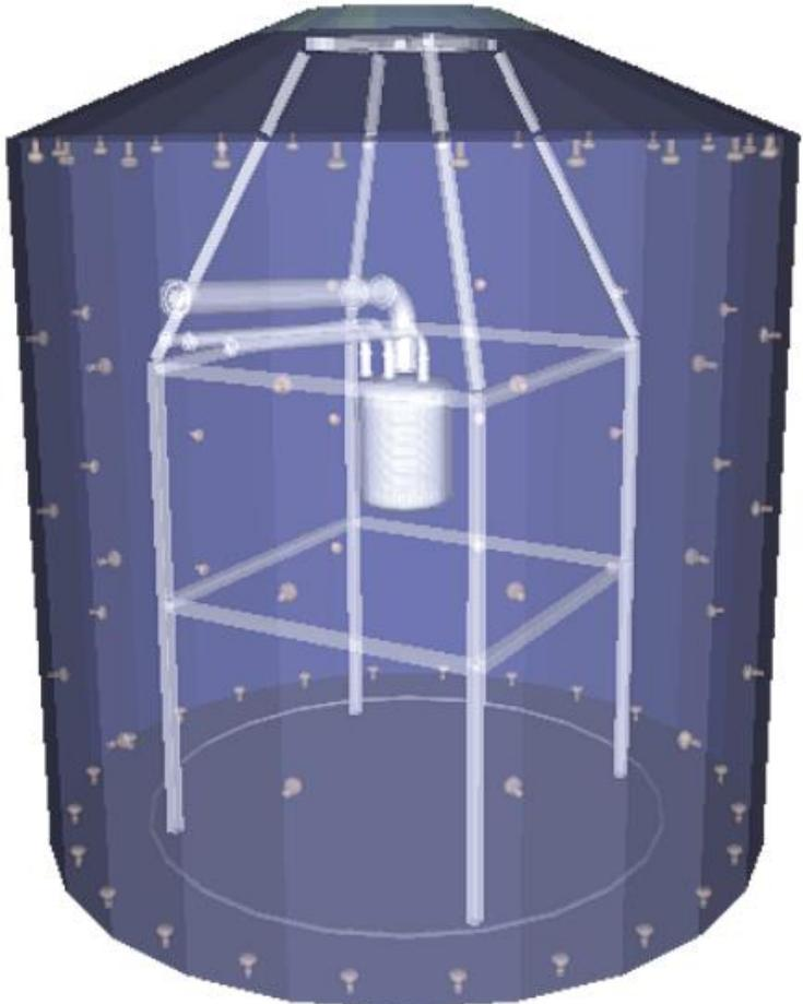
The XENON1T detector is hosted inside a **Muon Veto Water Tank**
