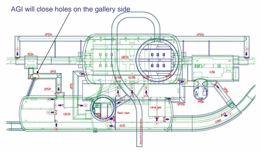
TS-EL to check that no Cu cable is missing in gallery Insulation should be applied between the cable duct and seal
