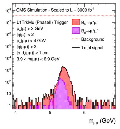
Low  $p_T$  dimuon trigger exploiting the capability of the upgraded CMS tracker.
