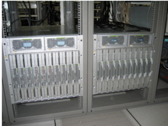
75 TB effective disk, 15 login machines, 38 batch nodes (152 CPU's)
