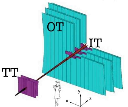
4-layer Silicon detector (0°, +5°, -5°, 0°), providing tracking before the magnet
