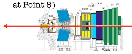
Direction of particles opposite to "natural" direction of LHCb detector
