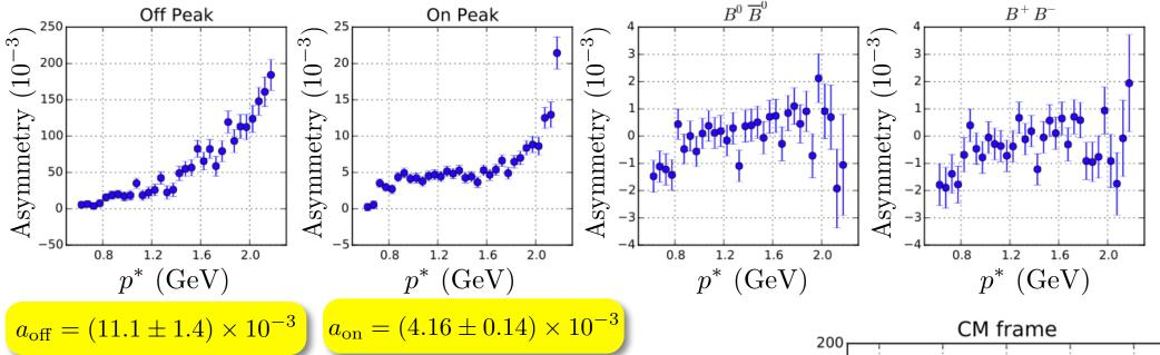
Larger off-peak asymmetry due to radiative Bhabha background and larger detector acceptance in backward (positron-beam) direction
