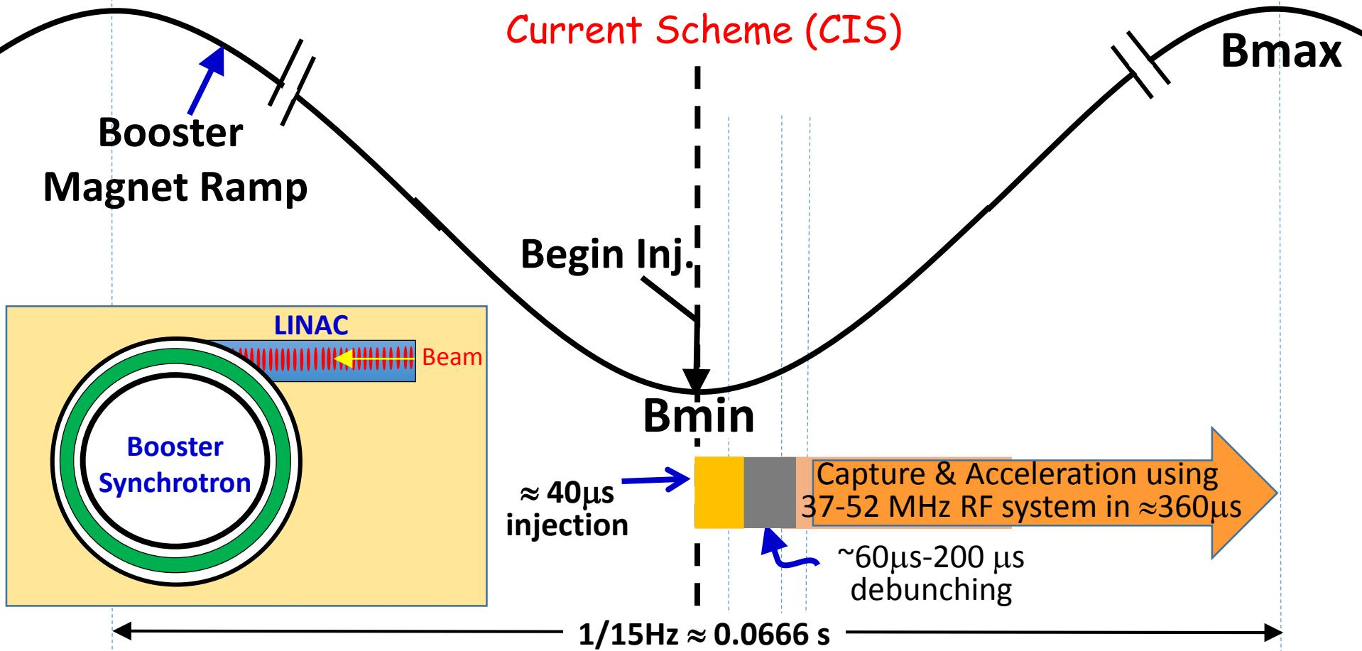
**Issues:** A limited time for Beam Capture & Acceleration. RF manipulations are non-adiabatic  $\leftarrow$  ~50% emittance dilution, 10% beam loss and large RF power
