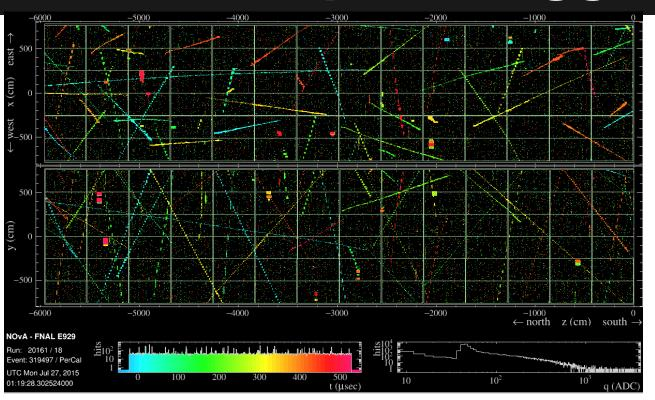
A 550 µsec exposure of the far detector showing the high rate of cosmic ray muons.
