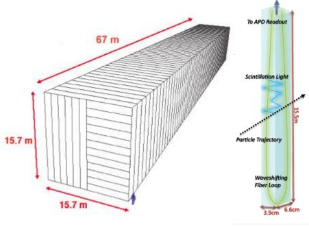
NOvA's alternating planes allow A NOvA cell particle tracking in 3D.
