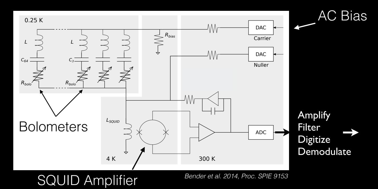
Readout 64 bolometers on single pair of wires using LC resonators to select an AC voltage bias
