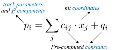
Finally, we apply a  $\chi^2$  cut to remove bad tracks, perform duplicate removal, and send all final tracks to LVL2 trigger.
