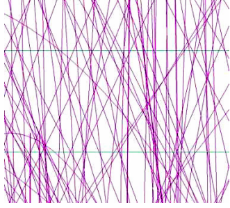
Figure 2: Track overlap in y-z plane (detector coordinates – see Fig. 3). 1cm layer separation is denoted by the two cyan lines. Note the significant overlap of tracks between these two layers, which will hinder tracker reconstruction.
