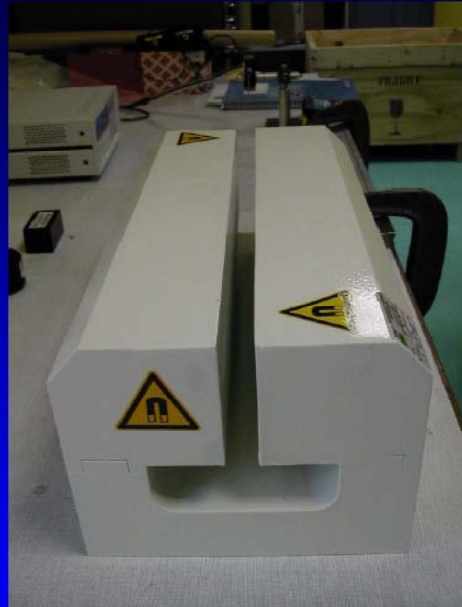
40 cm new magnet for GeV e beam
