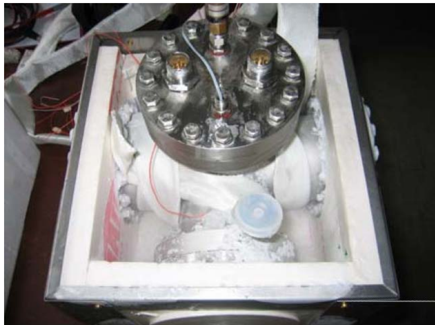
Chamber to study temperature dependence of fluorescence yield
