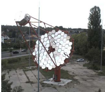
Figure 3: The baseline design for the 12 m diameter MST of Davies-Cotton type, with 8° FoV and 1500
