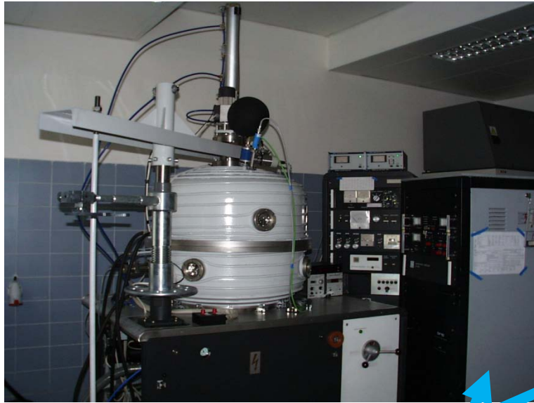
Aparature to deposit reflective and protective layers (Olomouc lab)
