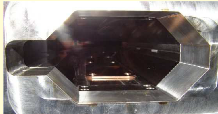
Electrode for e-cloud mitigation installed inside the dipole vacuum chamber
