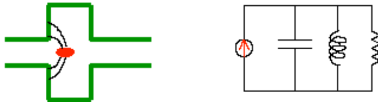
Fig. 2: RF cavity and the equivalent RLC parallel circuit model driven by a current generator.
