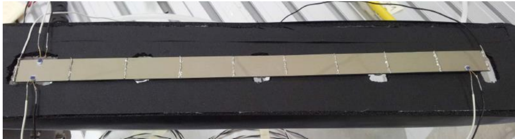
Stave equipped with dummy sensors (heaters)
