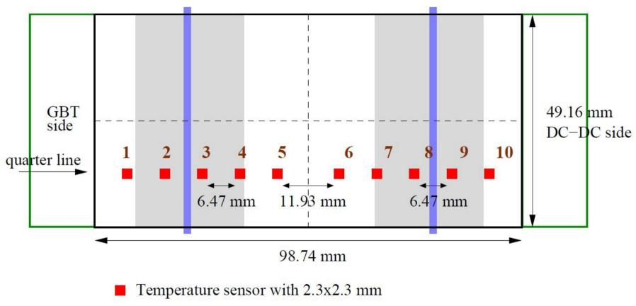
Sensor spacing on quarter line: 8.5 mm, first one at 7.5mm
