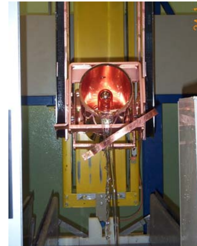
chemical Treatment of a quarter-wave resonator
