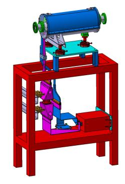
Engineering model of the prototype quadrupole magnet incl. support
