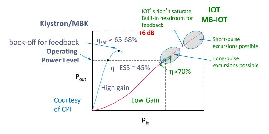
**Back-off for feedback, cost: 30%**  $\rightarrow$  Klystrons:  $\rightarrow$  IOTs: **Operate close to max efficiency**
