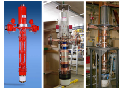
Fig. 1. Commercial 10 MW L-band MBK klystrons, left to right: Thales TH1501, Toshiba E3736 and CPI VKL-8301.
