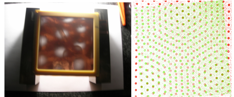
Figure 3.5: Left: Optical transparency of two standard GEM foils. Right: Illustration of the interference pattern that occurs when the foils are slightly rotated.
