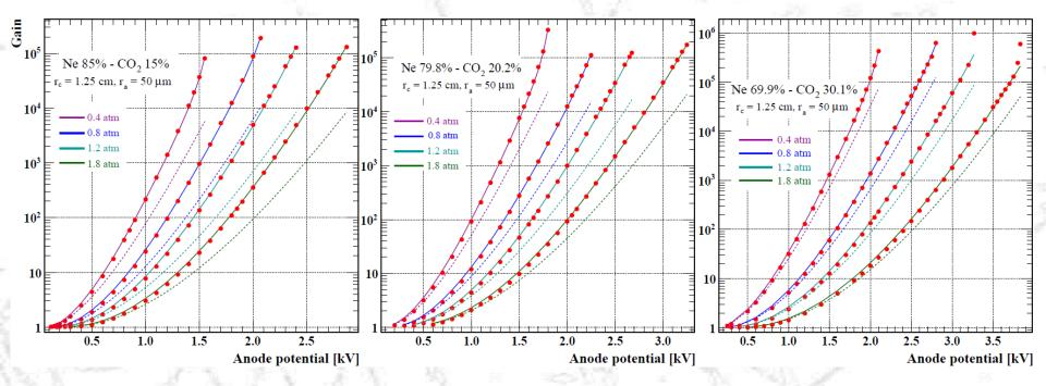
Energy transfers have more impact on gain (Penning effect) with increasing pressure and CO2 concentration,
