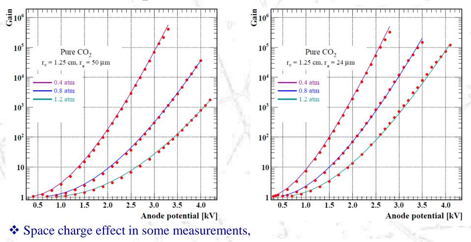
✤ Perfectly fine fits with all experimental gain curves; without any scaling or correction factor:
