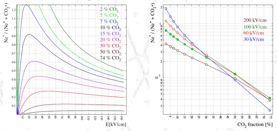
\* Effect of the excited Ne atoms to the total ionisation becomes significantly small at high  $CO_2$  percentages (left plot) and at high e-fields (right plot):
