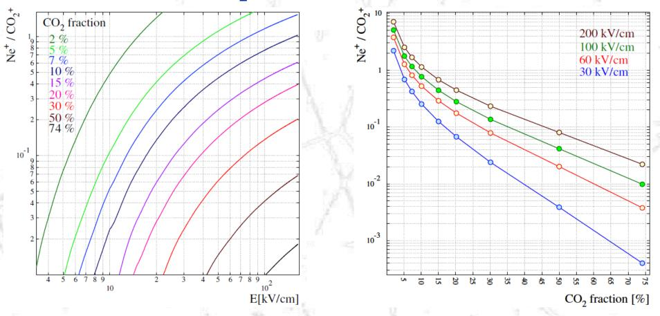
\* Most of the electron energy is picked up to ionise  $CO_2$  molecules because of the high ionisation cross section for  $CO_2$ ,
