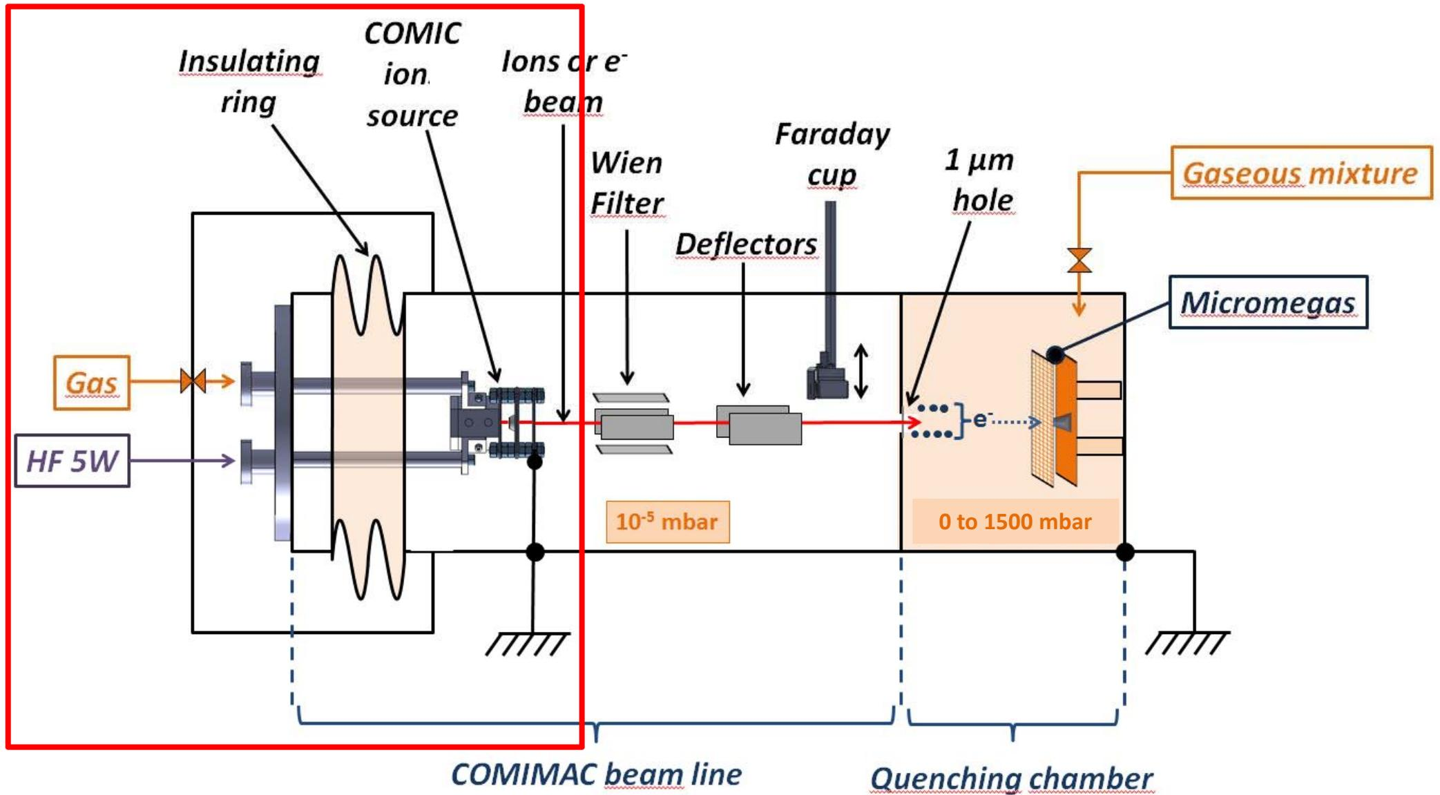
COMIC "**CO**mpact **Mi**crowave **CO**axial" is an highly optimized and miniaturized Electron Cyclotron Resonance (ECR) source developed at LPSC by SSI Group. (Patent: WO2010043831(A1)-2008)
