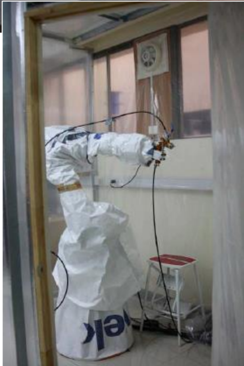
2. Chile: KUKA robot will be used for graphite spraying for module-0, can also used for X-ray testing completed chambers (gain uniformity)
