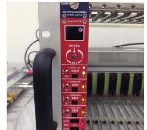
CAEN N1471H 50 pA current resolution. Labview controllable
