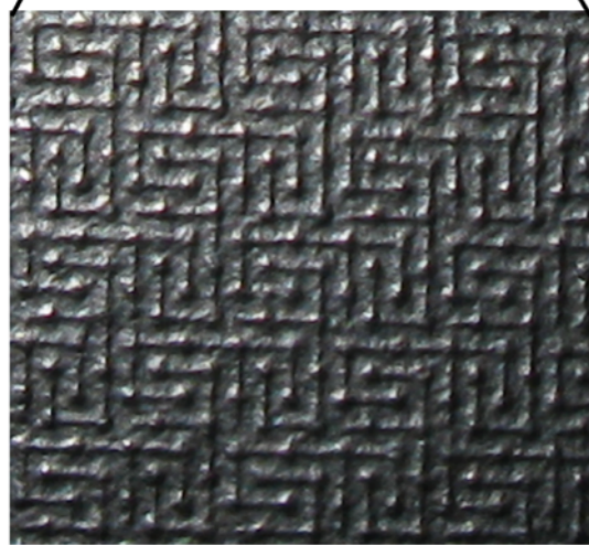
5 Mohm/sqr Kapton resistive layer. 25 um thick.
