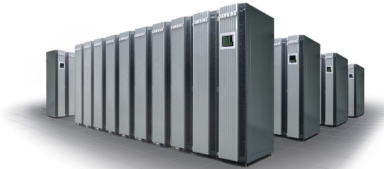
Dawning4000-A, 2004 AMD Opteron Grid-enabling Cluster 11.2 Tflops Peak
