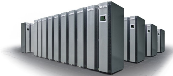
Dawning4000-A, 2004 AMD Opteron Grid-enabling Cluster 11.2 Tflops Peak
