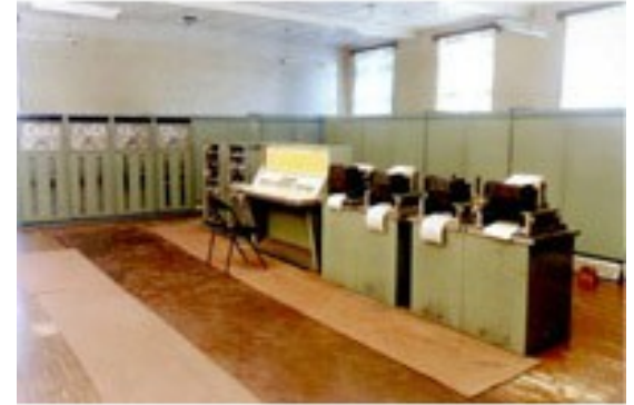
Model 109C First Large-scale Transistor Computer in China
