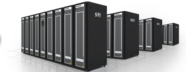
Dawning5000-A, 2008 6400 AMD 4-core Opteron 220 Tflops Peak
