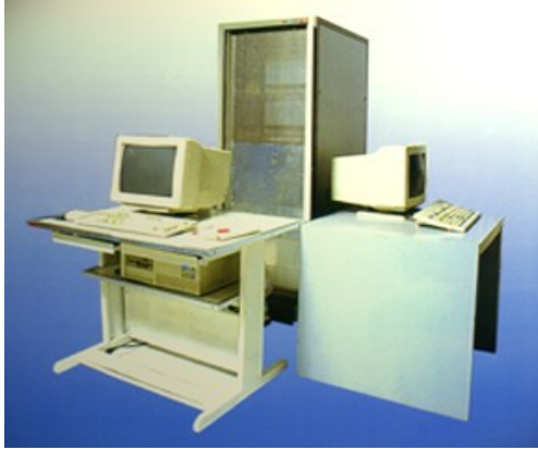
Dawning1000, 1995 intel i860 First MPP Computer in China 2.5Gflops Peak
