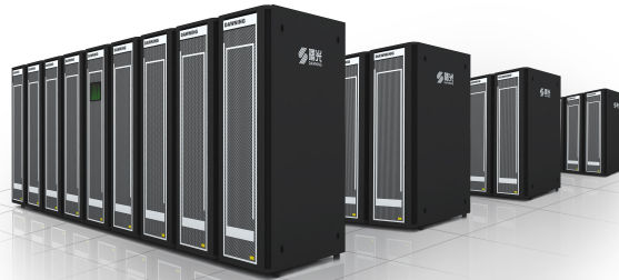
Dawning5000-A, 2008 6400 AMD 4-core Opteron 220 Tflops Peak
