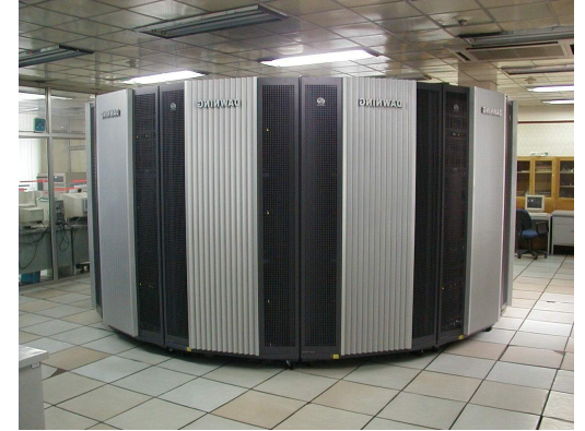
Dawning3000, 2001 IBM Power3 SUMA Cluster in China 400Gflops Peak
