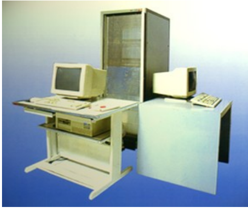
Dawning1000, 1995 intel i860 First MPP Computer in China 2.5Gflops Peak
