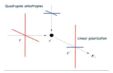
• Only quadrupole anisotropies generate polarization
