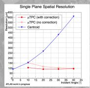
Combination of centroid &  $\mu TPC$  provides spatial resolution  $<100\,\mu m$  independently of the track incident angle!
