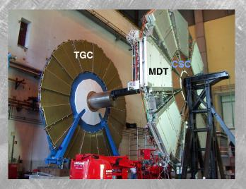
The current SW during the assembly phase. The 3 different detector technologies are visible.
