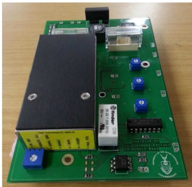
HV board for Prometeo.
