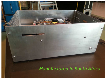
Prometeo mechanical enclosure.
