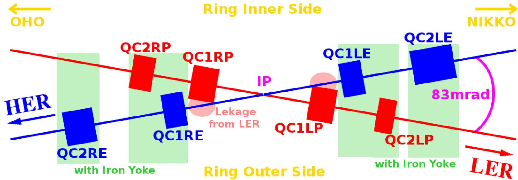
IR length of 8 m is sliced by 1 cm solenoids with dipole and gradient (rotated and shift) and nonlinear kicks (up to 21<sup>st</sup> multipole order) including quadrupole fringe field and kinematic term
