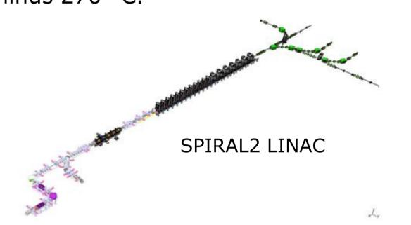
Why? In order to conduct electricity without resistance, the LINAC's electro magnets are cooled down to cryogenic temperatures.
