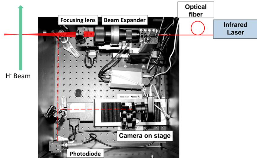
Laser Focus setup & Laser Diagnostics
