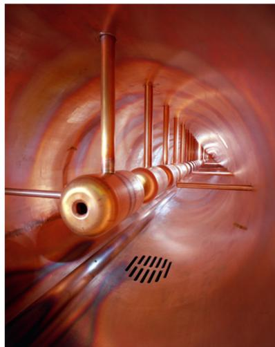
LINAC4 is a 80 m long linear accelerator currently in commissioning. It will be the first acceleration stage for hydrogen ions towards the LHC.
