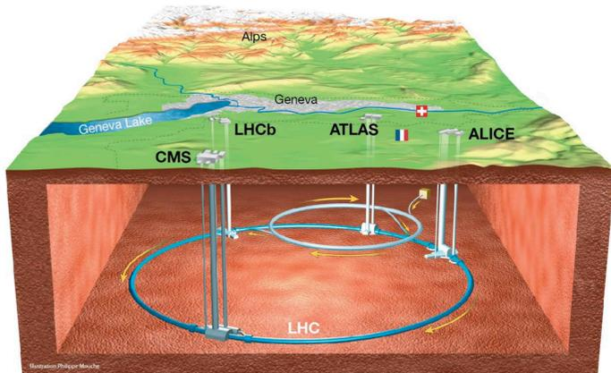
The 27 km long tunnel of the LHC, with its experiments and the preaccelerators. LINAC4 is situated right after the source of the particles which will be used at the LHC.
