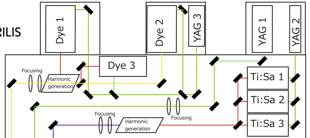
RILIS (Resonance Ionization Laser Ion Source) is the most element-selective and most common ion source used at ISOLDE. The technique is based on a multi-step resonance photo-absorption, using from two to four different laser beams from tuneable lasers (Dye and/or Ti:Sa lasers).
